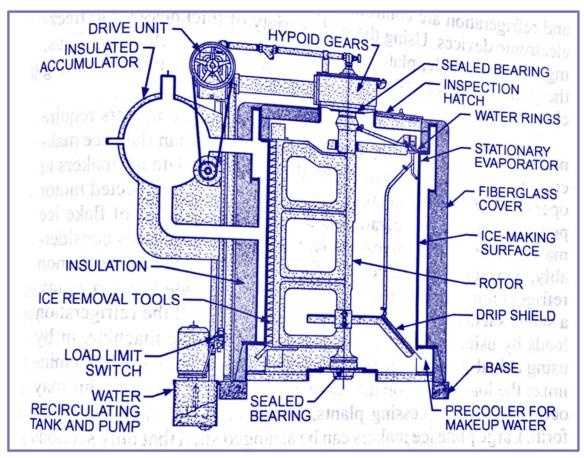
Thickness of ice produced by flake ice machines can be varied by adjusting the speed of the rotating part of the machine, varying evaporator temperature, or regulating water flow on the freezing surface. Flake ice is produced continuously, unlike to tubular and plate ice, which are produced in an intermittent cycle or harvest operation. The resulting thickness ranges from 0.04 0 .18 inches.
