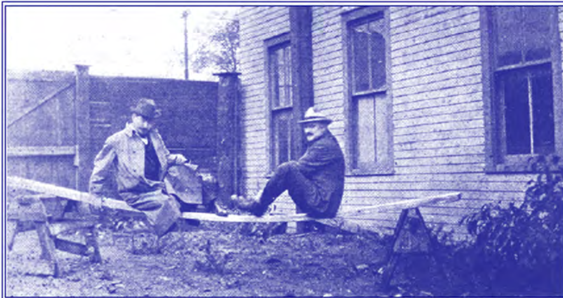
In 1917, the Journal of The American Society of Refrigerating Engineers reported tests to determine the elastic deformation of balsa wood. They were part of a study on the properties of balsa as an insulation material.
